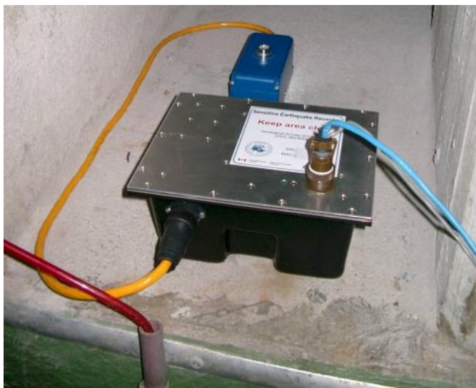
Figure 1. IA-1 with the external sensor, installed at the basement of the SIA building.
