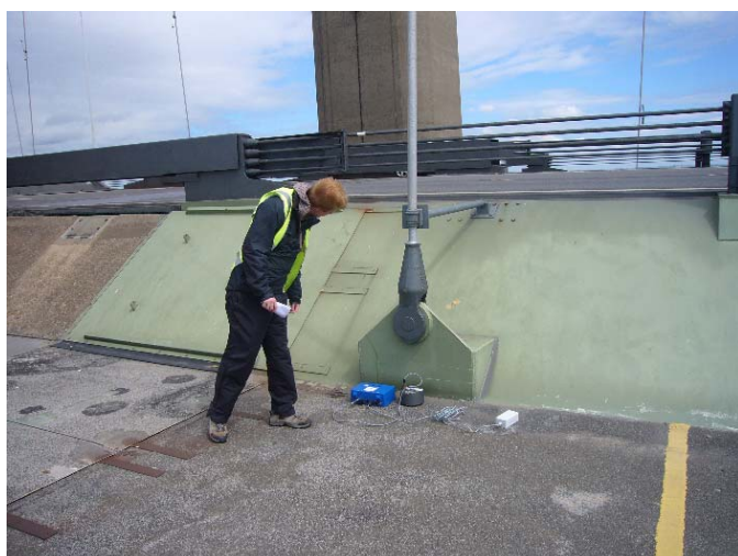
Figure 8. Checking recorder while measuring relative motion across the tower bearing
